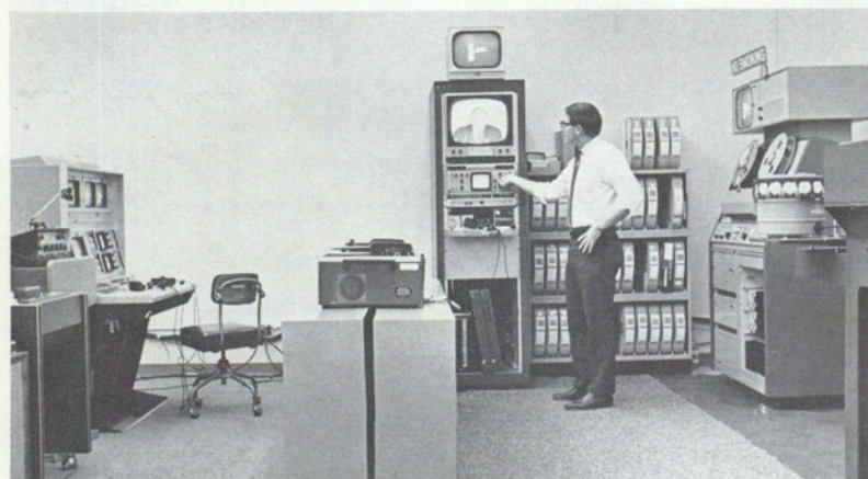
MASTER CONTROL AREA resembles that of commercial television station. Behind CHUCK KING are master tapes from which duplicate recordings are made for playback by field personnel.
